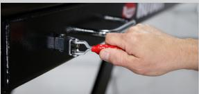
For fine platform positioning, release the four red handled swivel locks on both sides of the lift table allowing the tabletop to move freely. Re-engage locks when fine positioning is not needed.
