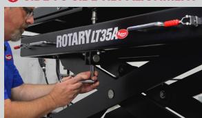
Use a 14mm or 9/16" socket or wrench on tilt mechanism located on the right side of the lift table to raise or lower platform +/-3°.
