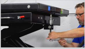
Adjust the tabletop with the object being removed or installed +3°/-1°. Tighten to raise the side with the tilt mechanism and loosen to lower it by using a 14mm or 9/16" socket or wrench.
